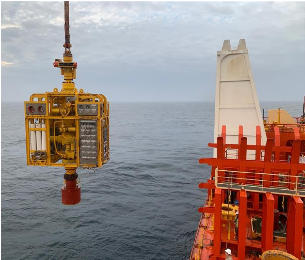
Deploying mechanical well control package
