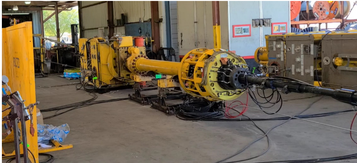
Dynamic testing of PCH with wireline
