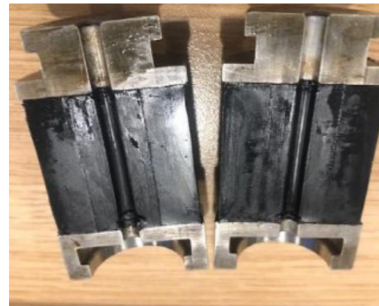
Packoff damage when RIH with diesel in bore
