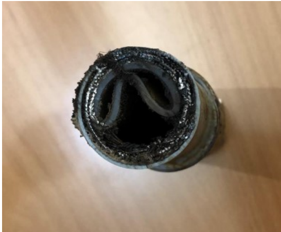
Collapsed circulation flying lead
