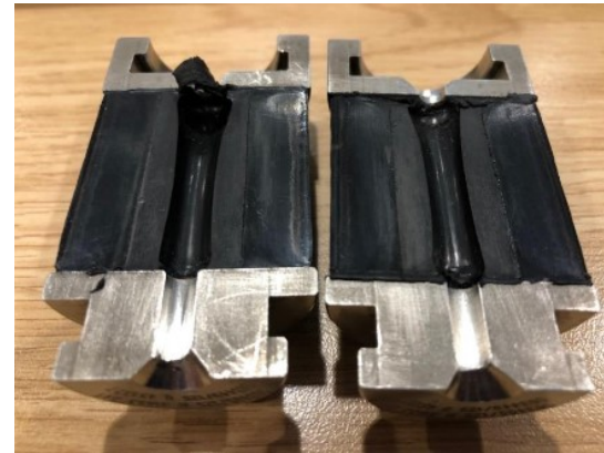
Packoff damage when RIH with diesel in bore
