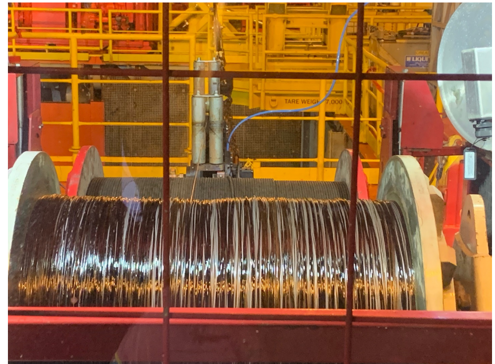
Asphaltenes deposited on slickline
