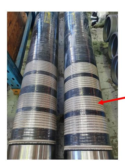
IPI developed DuraGrip™ surface fishing technology for Bi-directional anchoring and sealing without compromising packer integrity.
