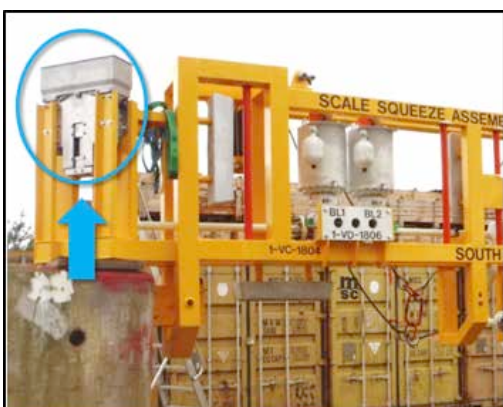
Figure 4: SECC female connector preinstalled on an extension frame prior to being attached to a manifold.
