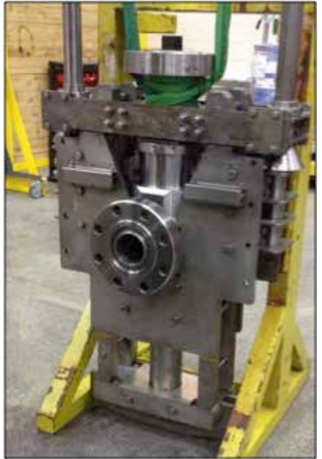
Figure 3: The four-inch connector in the mated position during factory acceptance testing.
