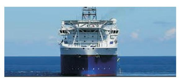
The Pride has underdeck carousel room for flexible and small-diameter rigid pipe-lay work, and a 7.2m x 7.2m moon-pool. The Pride can accommodate up to 100 people, in cluding marine crew. Accommodation is configured in single and double cabins.
