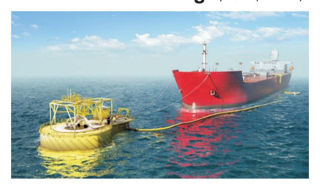
otal Upstream Production Nigeria (TUPNI) has praised NOV's Buoy Turret Loading System (BTL) concept, commenting that the "Egina OLT Buoy performed excellently during First Crude Lifting." With an average of 6000 m³/hour, the first offload of 1,000,000 barrels in just 28 hours went according to design and performance.
