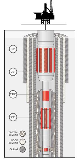
\*Also applicable for recovering 13 3/8" casing from inside 20" casing
